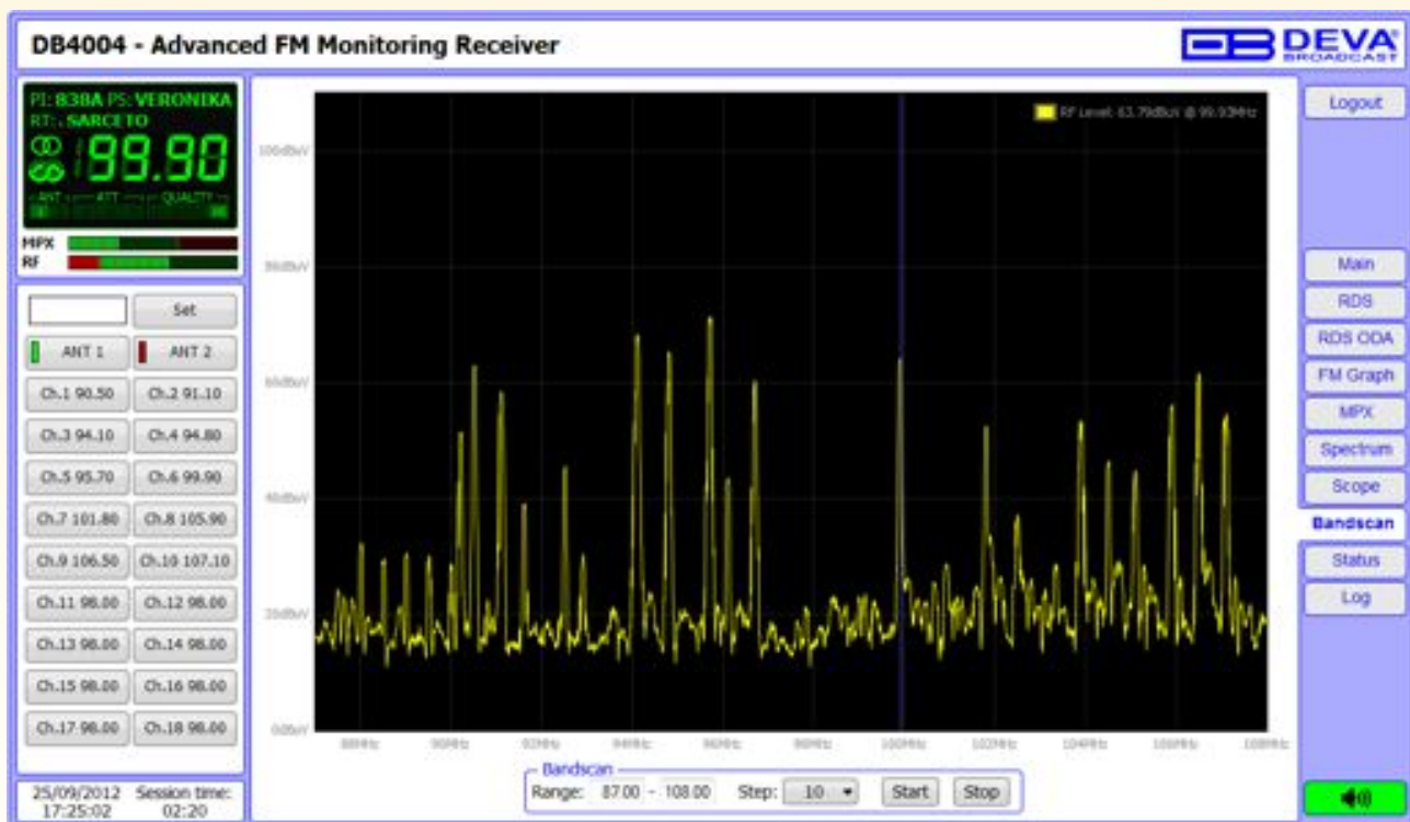
Band Analyzer presenting an overview of RF Level vs. the Frequency
