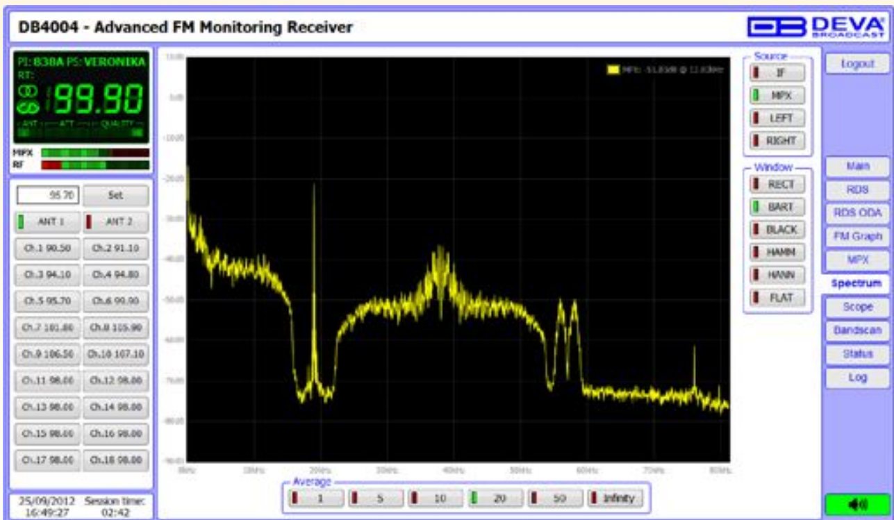
Spectral analysis of the MPX signal, determined on the basis of Fast Fourier Transform
