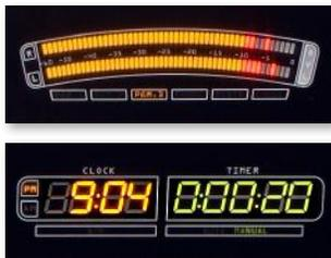
Radius has two dedicated meters for Program 1 and Program 2; the third is a "soft" meter that you can switch to meter Program 3, Program 4 / Phone / Record, or Monitor at the touch of a button.
